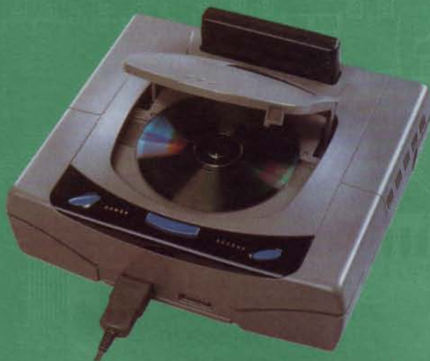
The Saturn's memory expansion slot enables future games to utilise extra ROM. So far, SNK is the only company to take advantage of this
